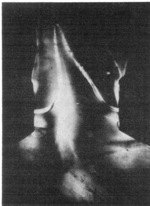
Figure 3 Crossed polar photograph showing discrete nature of core, seen when piston had been retracted after flow
