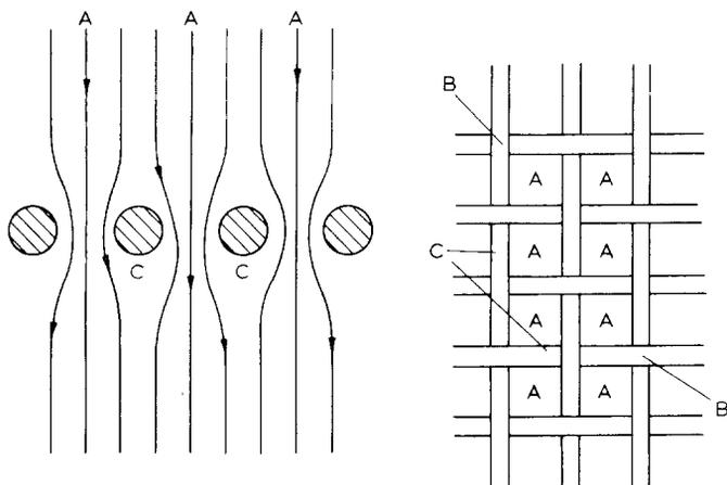
Fig. 3. Diagrammatic representation of laminar flow through a wire gauze
