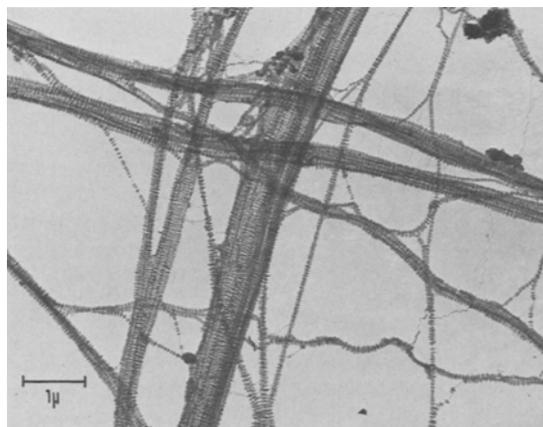
Fig. 2. Electron micrograph of shish kebabs crystallized and washed at  $T = 106^{\circ}\text{C}$
