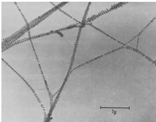
Fig. 1. Electron micrograph of shish kebabs crystallized and washed at  $T = 106^{\circ}\text{C}$
