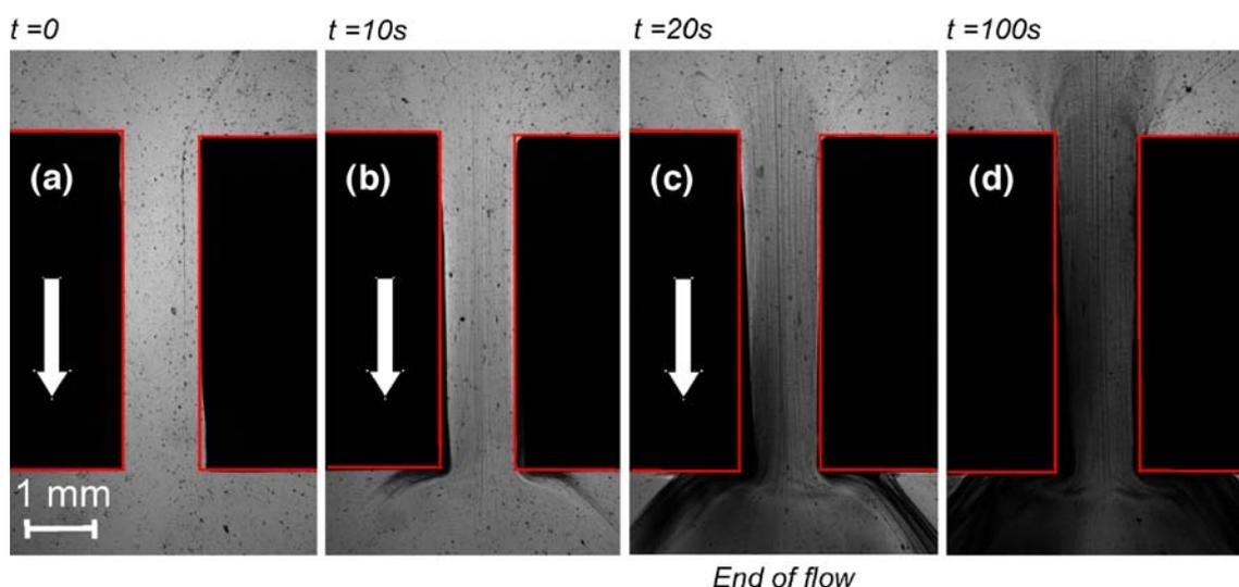
**Fig. 8** Development of FIC for HDPE in the shallow slit;  $T=130 \text{ °C}$ ; 0.5 mm/s piston speed,  $\dot{\gamma}_{app,w} \approx 290 \text{ s}^{-1}$  ( $We=63,000$ ). Optical observation in bright field. **a**  $t=0$  (before flow), **b** during flow, **c** end of
