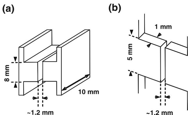
**Fig. 4** a The deep slit (depth, 10 mm) and b the shallow slit (1 mm)
