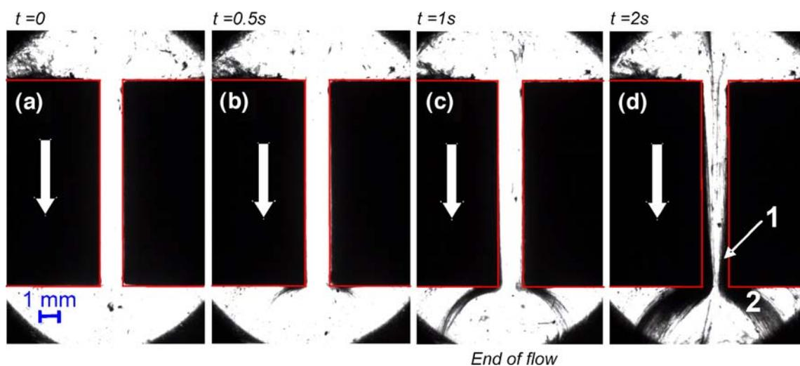
**Fig. 7** Development of FIC for HDPE in the deep slit;  $T=130\text{ }^{\circ}\text{C}$ ; 5 mm/s piston speed,  $\dot{\gamma}_{app,w} \approx 200\text{ s}^{-1}$  ( $We=40,000$ ). Optical observation in bright field. **a**  $t=0$  (before flow); **b**, **c** during flow; **d**  $t=2\text{ s}$  (end of flow). **1** Fibrous crystals generated at the wall, **2** downstream
