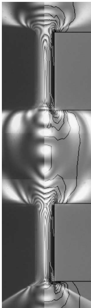
Fig. 5. Double-cavity flow birefringence patterns of the m-LLDPE at a temperature, 190^{\circ}\text{C} and flow rate, 33.9\text{ mm}^3/\text{s} (apparent wall shear rate in the slit \sim 44\text{ 1/s} ). Flow is from top to bottom. Comparison of the overall experimental flow birefringence pattern with the simulated PSD (the right hand part of the figure). As seen, the Wagner model simulations captured the fringe pattern at cavity 1 (mushroom shape) and cavity 2 (butterfly shape). The increment of PSD contour lines is 2.95 \times 10^4\text{ Pa} ( C, 1.74 \times 10^{-9}\text{ 1/Pa} ).
