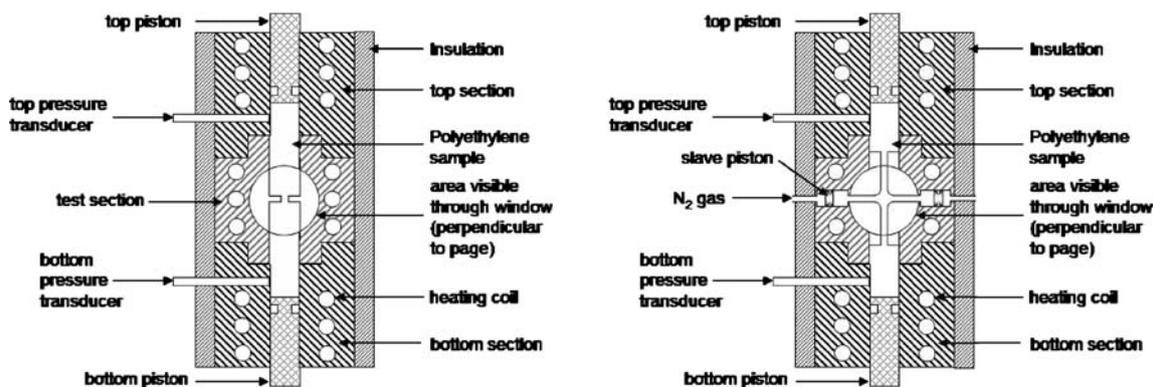
**Fig. 2** Schematic outlining the MPR design of (left) the contraction–expansion slit and (right) the cross-slot
