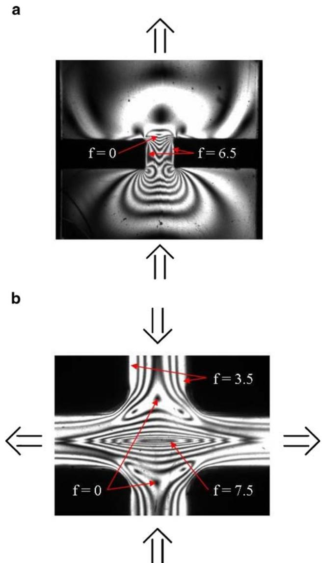
**Fig. 3** Stress-induced birefringence images taken at 155 °C. **a** Contraction–expansion, volumetric flow rate  $78.5 \text{ mm}^3 \text{ s}^{-1}$ , apparent wall shear rate within the slit  $\sim 24 \text{ s}^{-1}$ . **b** Cross-slot, volumetric flow rate through each channel  $34.5 \text{ mm}^3 \text{ s}^{-1}$ , wall shear rate  $\sim 9.2 \text{ s}^{-1}$ , maximum extension rate  $\sim 3.8 \text{ s}^{-1}$
