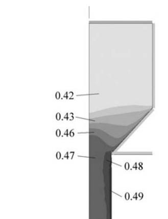
Figure 8. Spatial distribution of liquid fat content in chocolate during an axisymmetric extrusion ( $D_0/D = 15:5$ ,  $L = 0$ ,  $\alpha = 45^\circ$ ).
