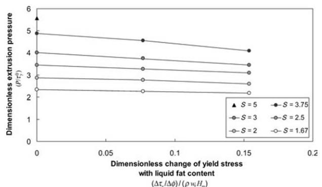
Figure 12. Extrusion pressure as a function of yield stress dependence on liquid fat content for different diameter reductions  $s = D_0/D$ .
