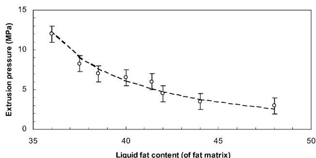
Figure 4. Extrusion pressure as a function of initial liquid fat content for a particular extrusion die geometry ( $D_0/D = 15 \text{ mm} : 4 \text{ mm}$ ,  $L/D = 4 \text{ mm}$ ,  $\alpha = 45^\circ$ ). Extrusion pressure data from Ovaici (1999).
