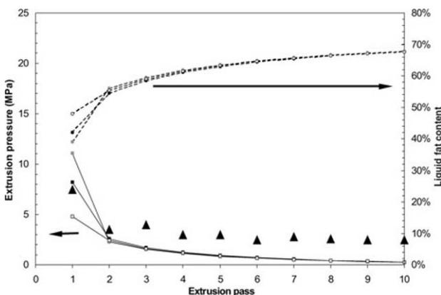
Figure 11. Sequence of extrusion pressures and corresponding liquid fat contents at the beginning of each extrusion pass. Circles/dashed lines correspond to three different evolutions of liquid fat (depending on the starting value), squares/solid lines to the evolution of extrusion pressure for the same starting values of liquid fat content and triangles to an experimentally observed extrusion pressure sequence.
