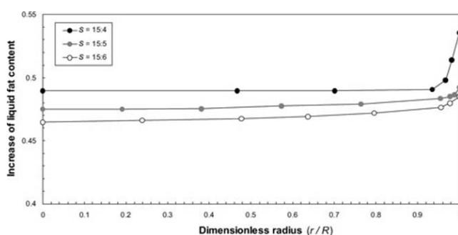
Figure 9. Change of the liquid fat content from the initial value to its value in the exit plane of axisymmetric orifice dies as a function of radial position. Plotted for three extrusion dies with different area reductions  $s = D_0/D$ .
