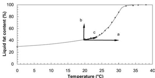
Figure 5. Liquid fat content as a function of temperature with three possible process paths for extrusion processing of semi-solid chocolate.
