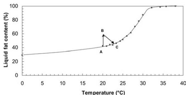
Figure 6. Liquid fat content as a function of temperature with suggested process path for extrusion processing of semi-solid chocolate.
