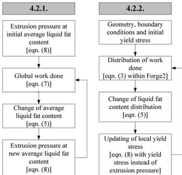
Figure 10. Calculation procedures for change in extrusion pressure as an effect of the change in liquid fat content (for a sequence, respectively a single extrusion).
