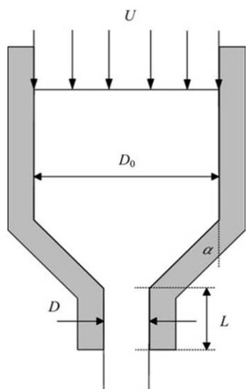
Figure 1. Axisymmetric extrusion geometry.
