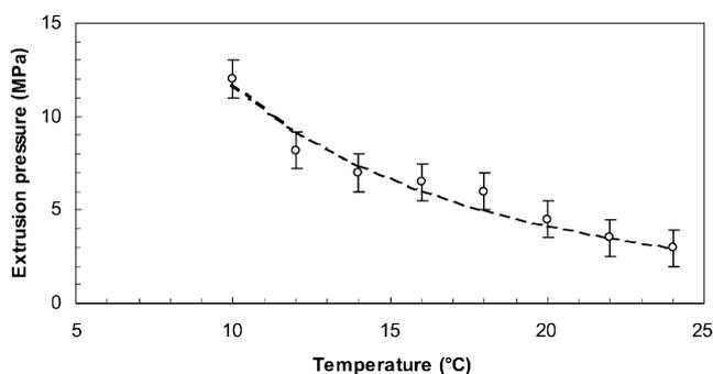
Figure 2. Extrusion pressure as a function of initial temperature for a particular extrusion die geometry and flowrate ( $D_0/D = 15 \text{ mm}/4 \text{ mm}$ ,  $L/D = 4 \text{ mm}/4 \text{ mm}$ ,  $\alpha = 45^\circ$ ,  $Q = 5 \times 10^{-7} \text{ m}^3 \text{ s}^{-1}$ ). Data replotted from Ovaici (1999).
