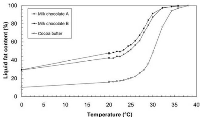
Figure 3. Dependence of liquid fat content with temperature, for two different milk chocolate compositions and a cocoa butter, as measured by pulsed nuclear magnetic resonance (p-NMR).
