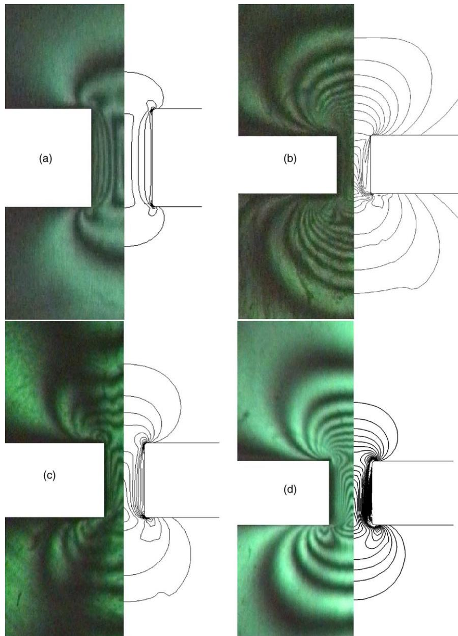
Fig. 8. Comparison of experimental birefringence with principal stress difference contour prediction made by Polyflow using the Wagner model for polystyrenes at 200 °C; (a) monodisperse Dow PS1569, piston speed 0.2 mm/s; (b) monodisperse Dow PS1571, piston speed 0.1 mm/s; (c) Durham 90%/10% 485k/66k PS blend, piston speed 0.2 mm/s; (d) polydisperse Dow PS680E, piston speed 2 mm/s.
