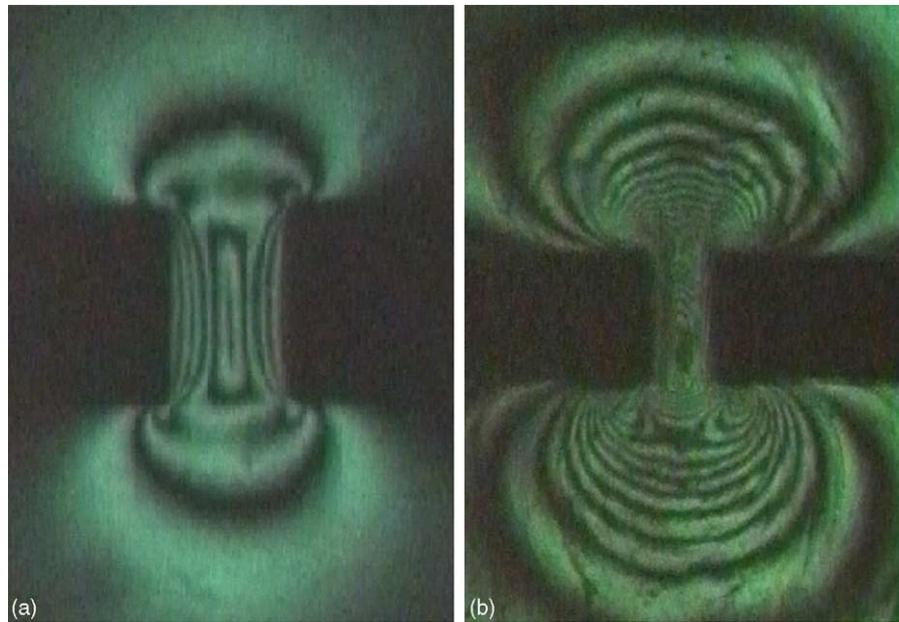
Fig. 3. Example flow birefringence of monodisperse polystyrenes at 200 °C; (a) slow flow ( $We \approx 1$ ): PS1569, piston speed 0.2 mm/s; (b) intermediate flow ( $We \approx 50$ ): PS1571, piston speed 0.1 mm/s.
