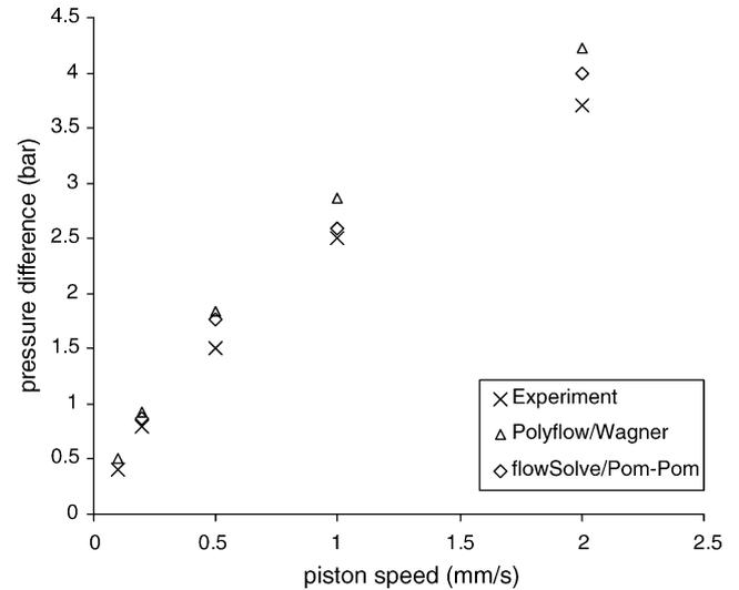
Fig. 9. Comparison of experimental pressure difference with predicted values for PS680E at 200 °C.
