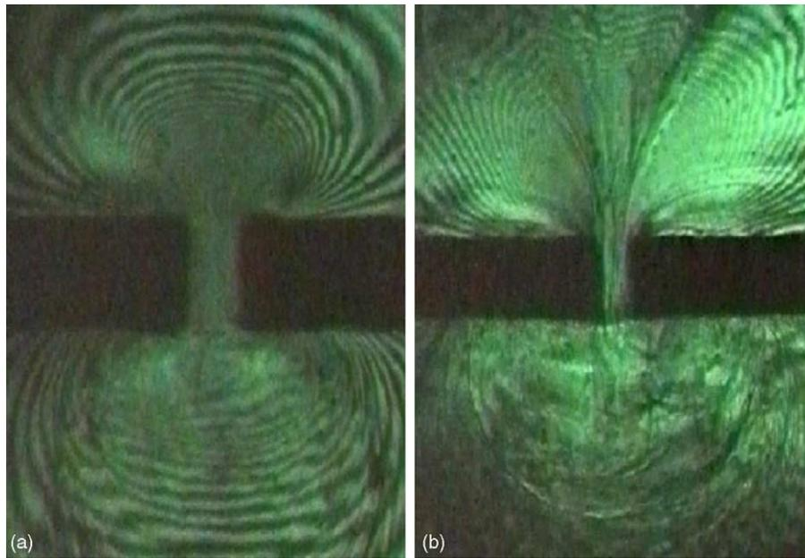
Fig. 5. Flow birefringence of PS1571 at 200 °C; (a) pulsing instability, piston speed 0.5 mm/s; (b) viscoelastic disturbance, piston speed 2 mm/s.
