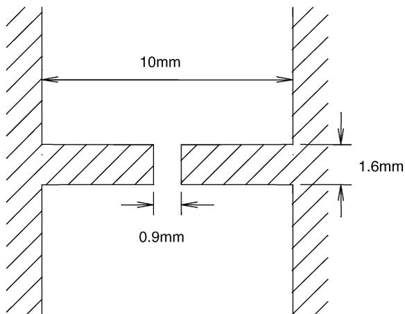
Fig. 2. MPR slit flowcell geometry.
