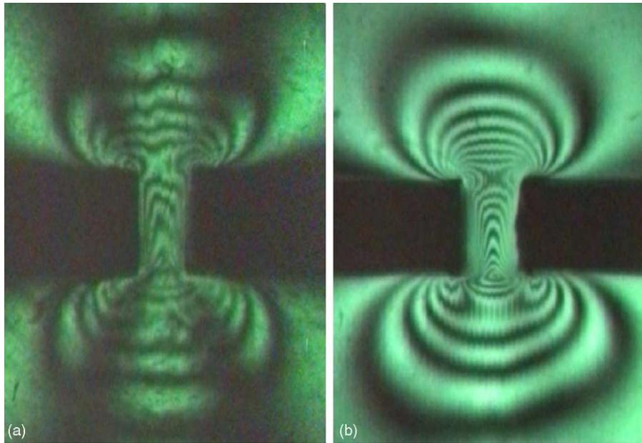
Fig. 7. Example flow birefringence of bimodal blend and broadly polydisperse polystyrenes at 200 °C; (a) 90%/10% 485k/66k PS blend, piston speed 0.2 mm/s; (b) PS680E, piston speed 2 mm/s.
