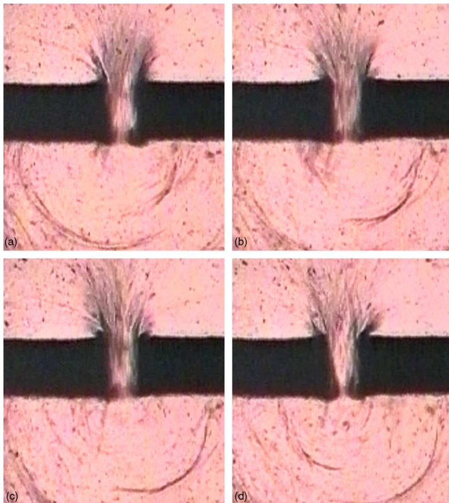
Fig. 6. Bright field observations of Dow PS1571 PS at 180 °C; piston speed 1.0 mm/s; time interval between frames (a)–(d) 0.2 s.
