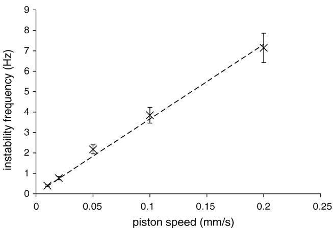
Fig. 4. Change in frequency of pulsing instability; Dow PS1571 at 180 °C.
