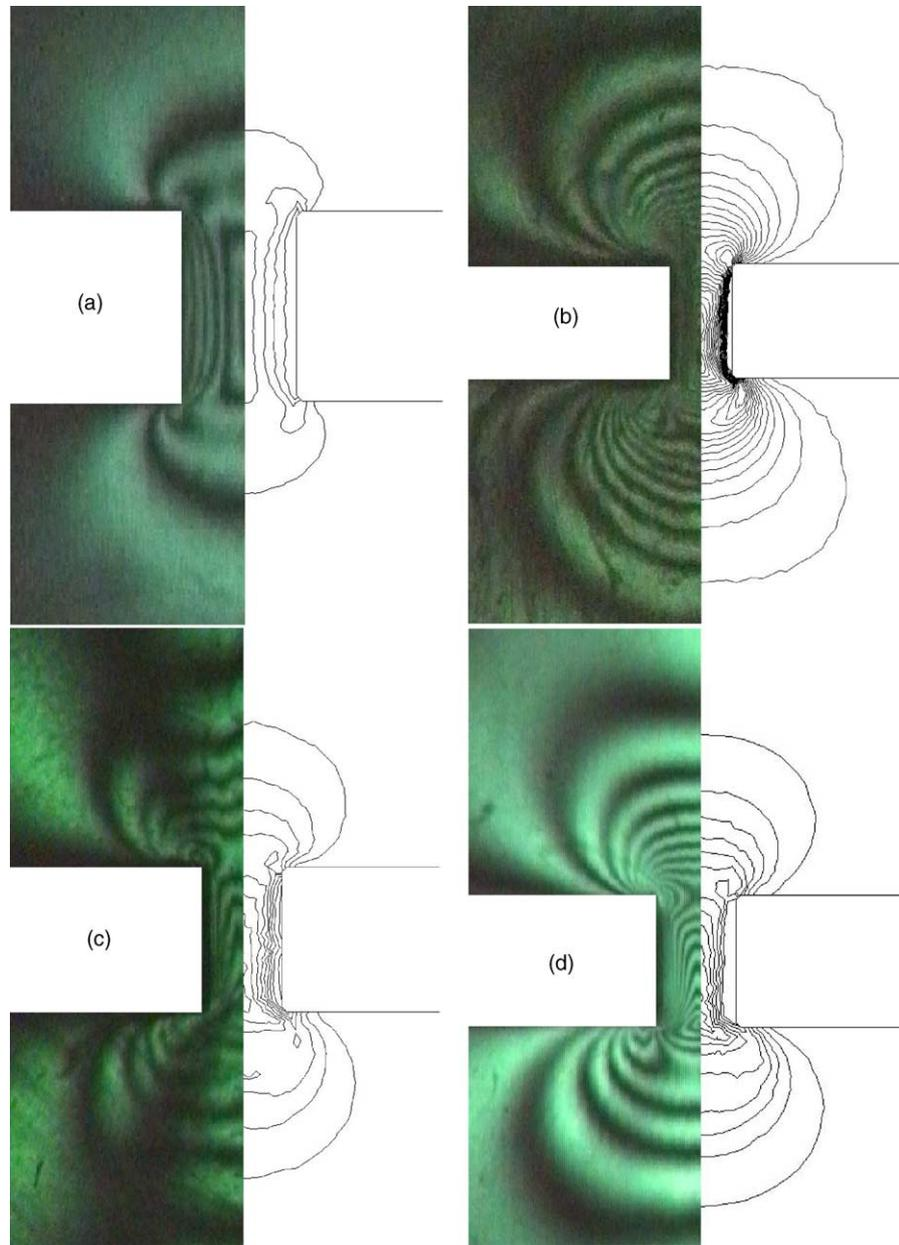
Fig. 10. Comparison of experimental birefringence with principal stress difference contour prediction made by flowSolve using the Pom-Pom model for polystyrenes at 200 °C; (a) monodisperse Dow PS1569, piston speed 0.2 mm/s; (b) monodisperse Dow PS1571, piston speed 0.1 mm/s; (c) Durham 90%/10% 485k/66k PS blend, piston speed 0.2 mm/s; (d) polydisperse Dow PS680E, piston speed 2 mm/s.
