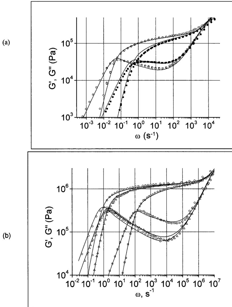
**FIG. 2.** Linear rheology of (a) 250k (filled symbols) and 485k PS (open symbols) melts and (b) PB 48 (squares), 156 (triangles), and 210k (circles) melts with comparison to predictions from the tube theory, parameterized by a chemistry- and temperature-dependent entanglement modulus  $G_e$  and Rouse relaxation time of an entanglement segment  $\tau_e$ , and the material dependent number of entanglements  $Z$ .
