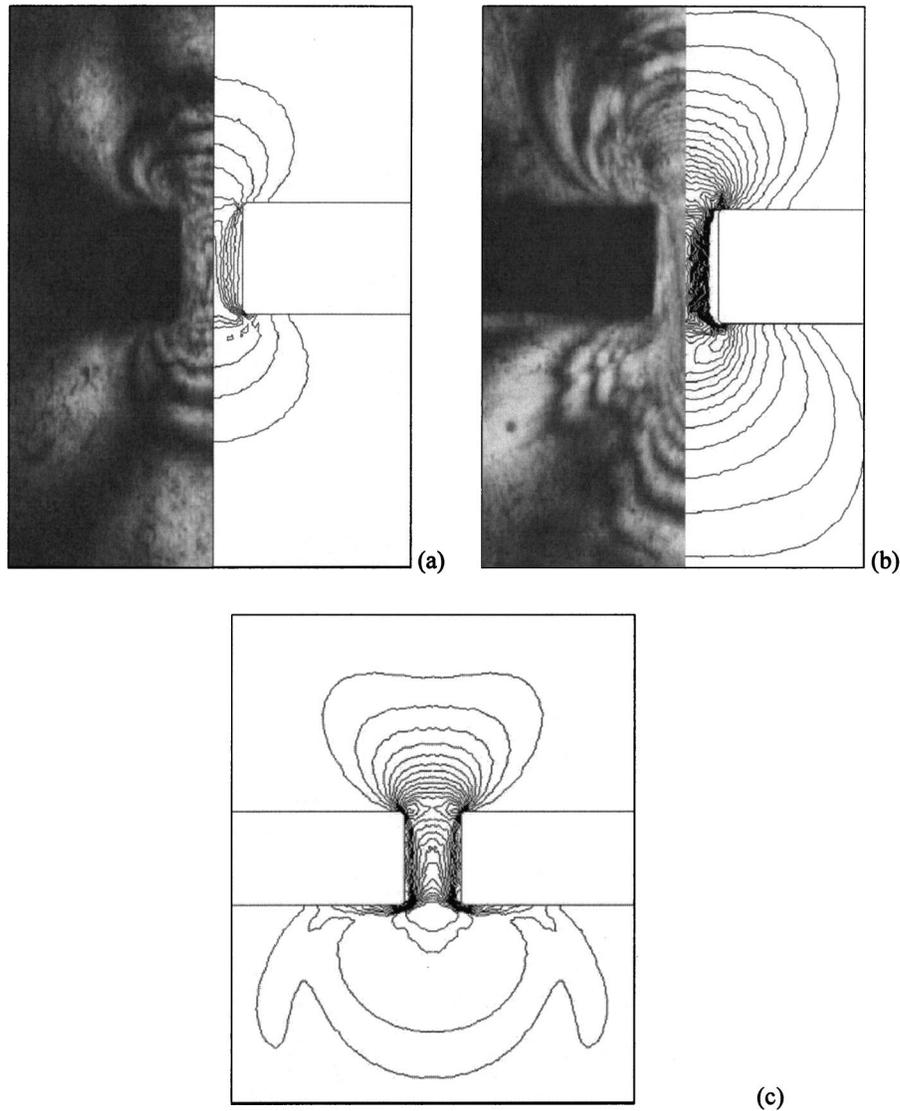
**FIG. 6.** Experiment and calculation of stress fields for the PS485 monodisperse melt. Piston speeds are (a) 0.05 mm/s, (b) 0.2 mm/s, (c) 5 mm/s, giving wall shear rates of (a)  $2.9 \text{ s}^{-1}$ , (b)  $12 \text{ s}^{-1}$ , and (c)  $290 \text{ s}^{-1}$ . Flows (a) is in Regime (2), flow (b) on the threshold of regime (3) and (c) (calculated only) deeply into Regime (3).
