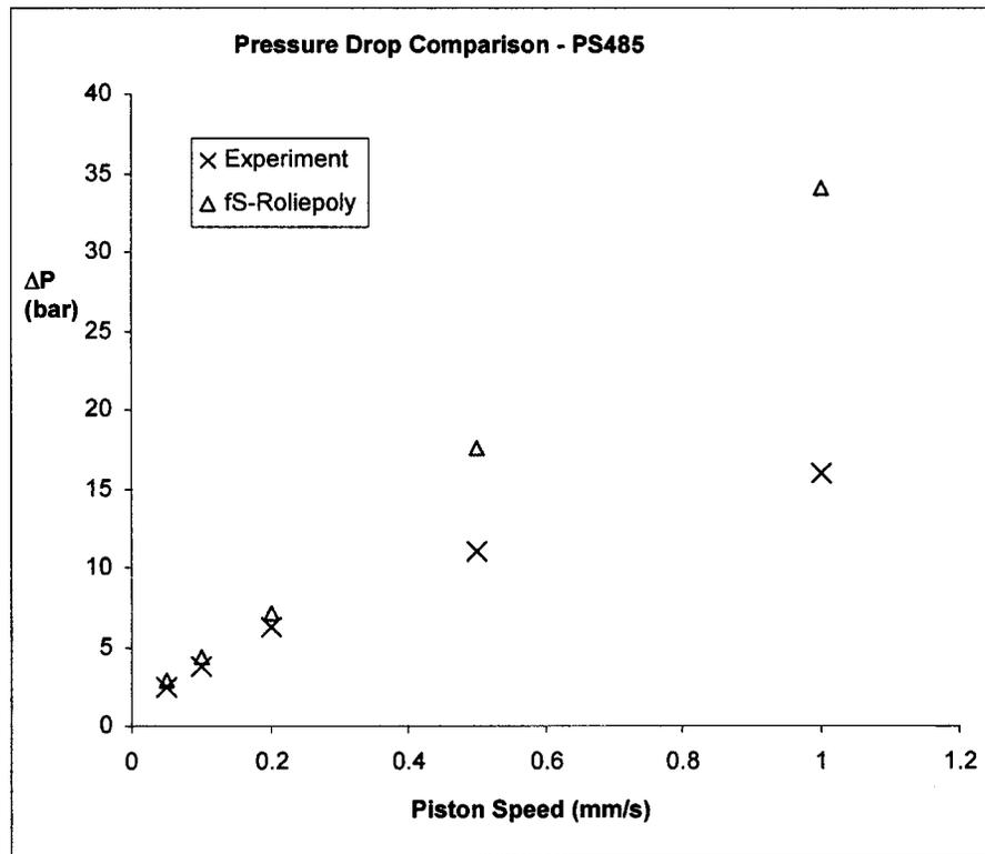
**FIG. 10.** Observed and simulated steady-state pressure drops as a function of piston speed for the PS485 melt. Above 0.5 mm/s (wall shear rate of  $29 \text{ s}^{-1}$ ), the observed values fall markedly below the predicted values, but this is also the regime in which the experiment showed flow instabilities, which are suppressed in the simulations.
