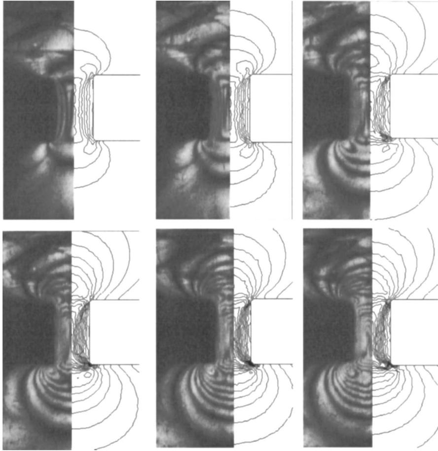
**FIG. 9.** PS262 K at 200 °C—Evolution of flow birefringence at piston speed of 0.5 mm/s (steady-state wall shear rate of  $29 \text{ s}^{-1}$ ): (a)  $t=0.25 \text{ s}$ , (b)  $t=0.5 \text{ s}$ , (c)  $t=0.75 \text{ s}$ , (d)  $t=1.0 \text{ s}$ , (e)  $t=1.25 \text{ s}$ , and (f)  $t=1.5 \text{ s}$  (fully developed).
