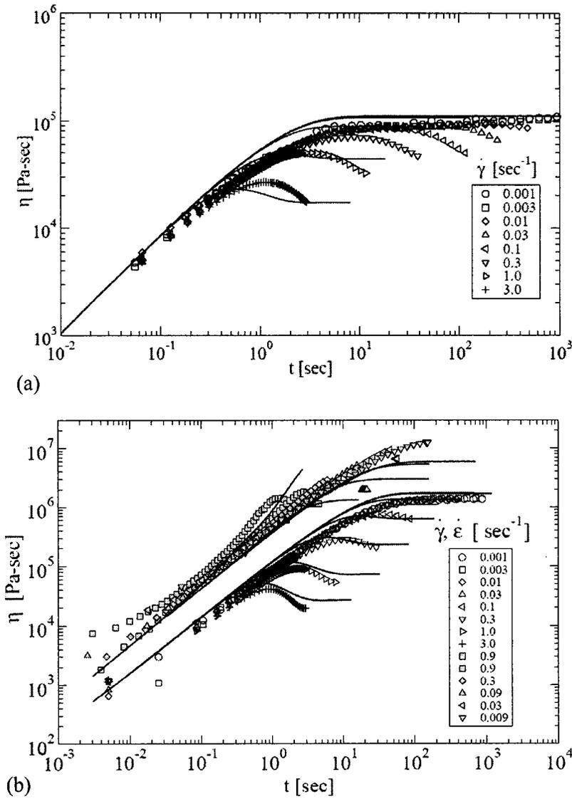
**FIG. 3.** Nonlinear shear and extensional (485k PS only) transients (rates from 0.01–3 s<sup>-1</sup>) rheology of 250k (a) and 485k PS (b) melts at 170 °C (the extensional data were time-temperature shifted from 160 °C). Comparison curves are predictions from the full tube theory of Eq. (2), parameterized by plateau modulus  $G_N^{(0)}$ , entanglement time  $\tau_e$ , and the number of entanglements  $Z$ .
