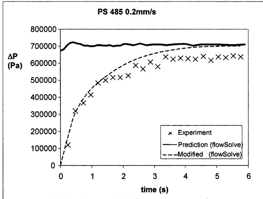
**FIG. 8.** Simulated (solid curve) and experimental data (crosses) on the pressure drop transient for flow start up in an 11:1 contraction of the PS485 melt at 170 °C. The effect of melt compressibility in the upstream piston is marked. The dashed curve shows the modified simulations of the pressure drop when the upstream boundary velocity condition was modulated with a single exponential growth.
