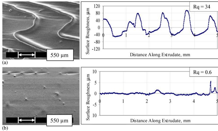
Fig. 18. SEM images and surface profilometry profiles with  $R_q$  values for extrudate surfaces of (a) HDPE and (b) HDPE + PPA extruded at 0.6 rpm and 190 °C through die A (note ordinate scale difference).
