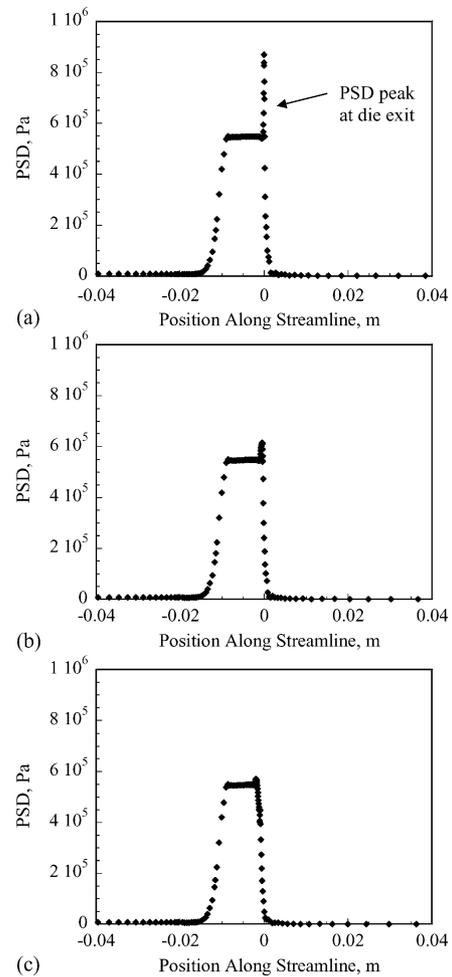
Fig. 7. PSD values along streamlines 50 μm from the die wall simulated in polyflow for the LLDPE at 190 °C through dies (a) A, (b) B and (c) C.
