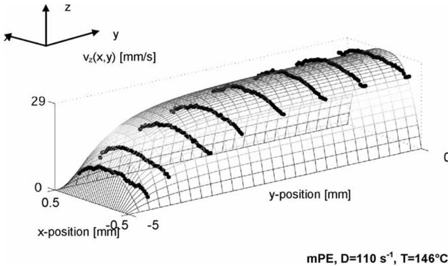
Fig. 20. Velocity profiles and matching numerical simulation in branch 2 region of flow for mPE (For details see Robert et al. [40])
