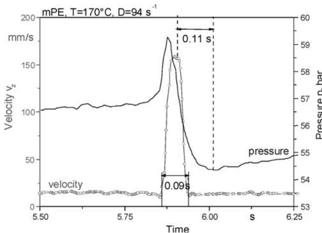
Fig. 18. Pressure and velocity fluctuations for mPE at  $z = 20$  mm (For details see Merten et al. [21])
