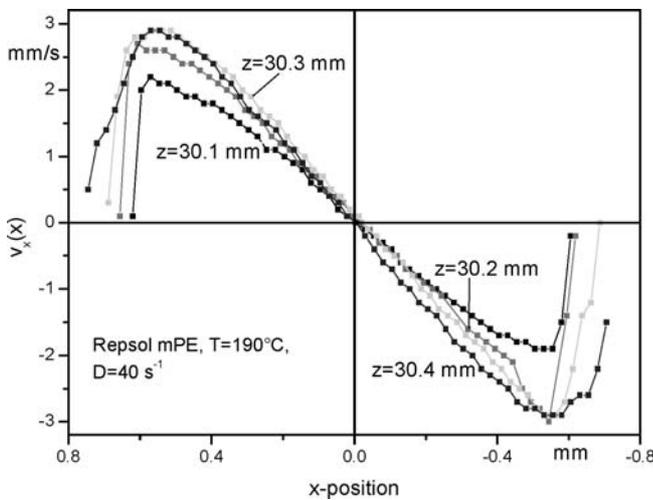
Fig. 7. Horizontal  $V_x$  velocity profiles for mPE flowing within and outside a slit die (For details see Merten [20])
