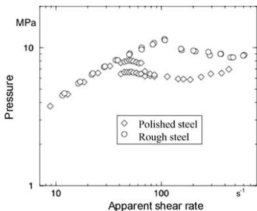
Fig. 26. Effect of surface roughness on flow curves (For details see Robert [38])
