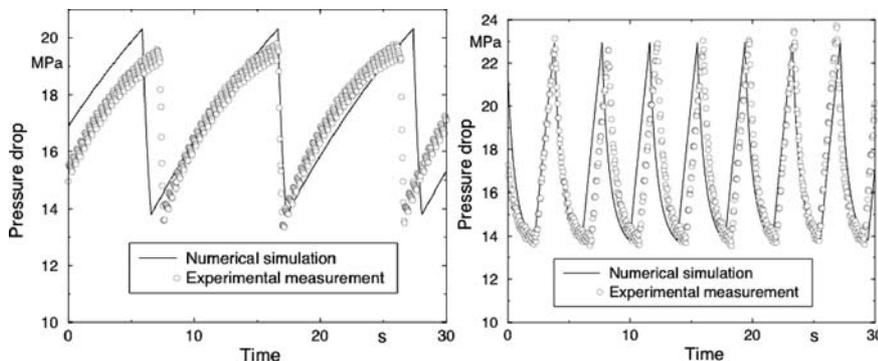
Fig. 24. Matching of pressure fluctuations in stick-spurt flow with model predictions (For details see Robert [38])
