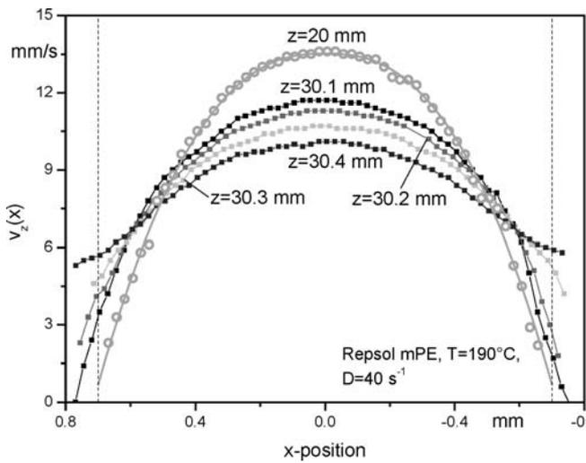
Fig. 6.  $V_z$  velocity profiles for mPE flowing within and outside a slit die (For details see Merten [20])
