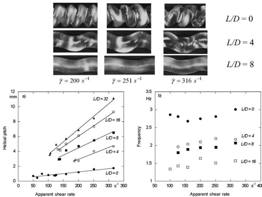
Fig. 28. The effect of apparent shear rate and  $L/D$  on volume instabilities for polystyrene (For details see Combeaud et al. [53])
