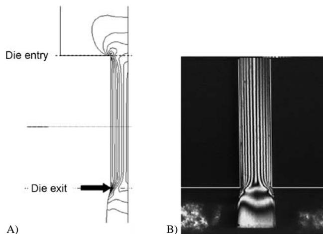
Fig. 4. Example of A) numerical simulation and B) experimental birefringence for LLDPE, illustrating stress concentration at exit of die (For details see Arda and Mackley [7])
