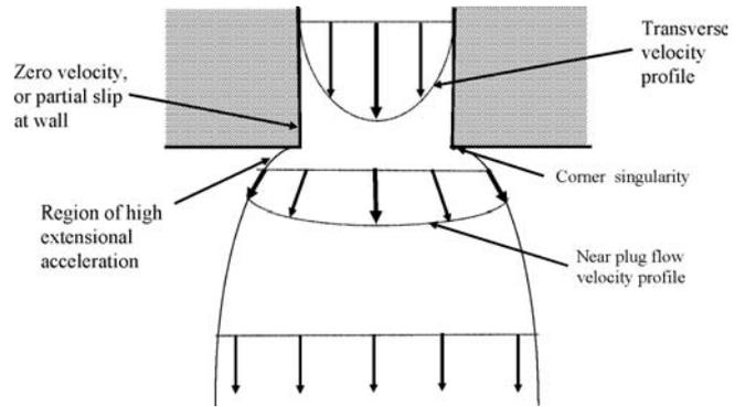
Fig. 8. Schematic diagram of velocity profile rearrangement at the exit of a slit die
