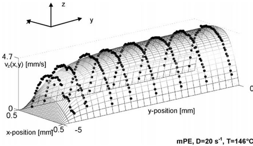
Fig. 19. Velocity profiles and matching numerical simulation in branch 1 region of flow for mPE (For details see Robert et al. [40])
