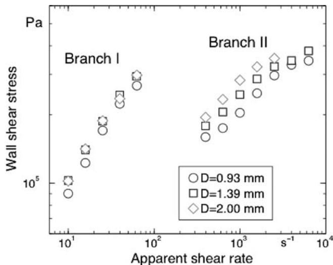
Fig. 16. Flow curves for mPE for different capillary diameters (For details see Robert [38])
