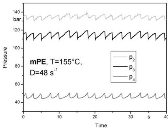
Fig. 17. Pressure fluctuations for mPE at three different positions within slit die (For details see Merten et al. [21])
