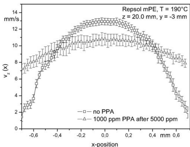
Fig. 14. Effect of additive on velocity profile at the slit die exit for mPE. PPA additive initially applied within polymer at 5000 ppm and subsequently at 1000 ppm (For details see Merten [20])
