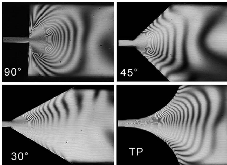
Fig. 31. FIB patterns for polystyrene in stable flow conditions for the different entrance geometries (For details see Combeaud et al. [72])
