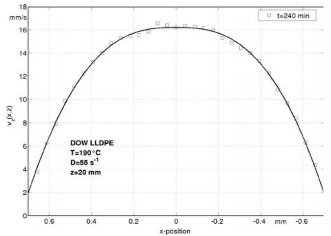
Fig. 9.  $V_z$  velocity profiles for LLDPE flowing at  $z = 20$  mm within the slit die (For details see Merten [20])
