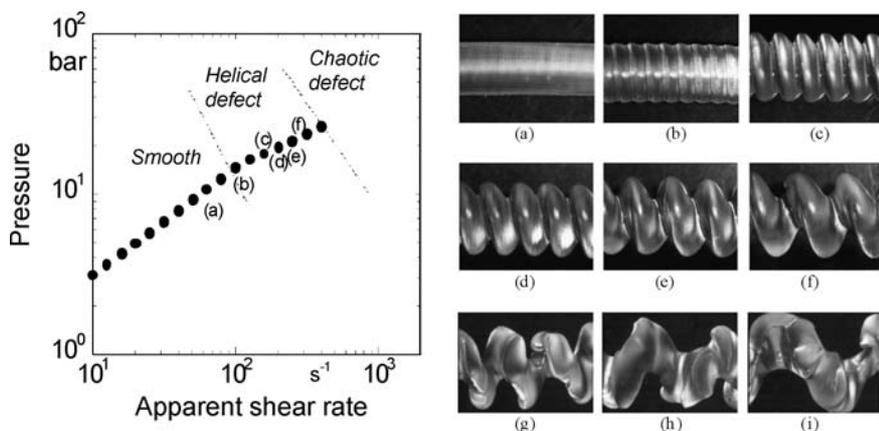
Fig. 2. Examples of upstream instabilities and associated flow curve (For details see Combeaud et al. [72])
