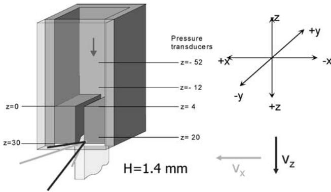
Fig. 5. Schematic diagram of optical slit geometry used in the “Erlangen” experiments. The slit  $z = 0$  mm position was taken at the entrance of the slit and the exit of the slit was at  $z = 30$  mm
