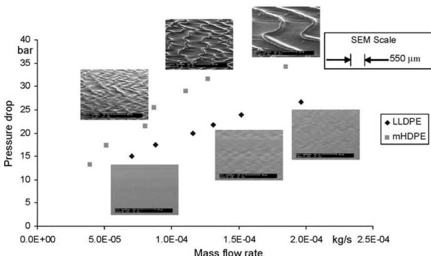
Fig. 10. SEM Photographs for LLDPE and mPE showing that the magnitude of the instability is greater for mPE than LLDPE at the same extrusion pressure drop (For details see Arda and Mackley [7])
