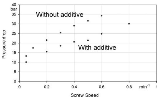
Fig. 13. Effect of additive on extrusion pressure drop for mPE without and with 1500 ppm fluoropolymer processing aid (For details see Arda and Mackley [7])
