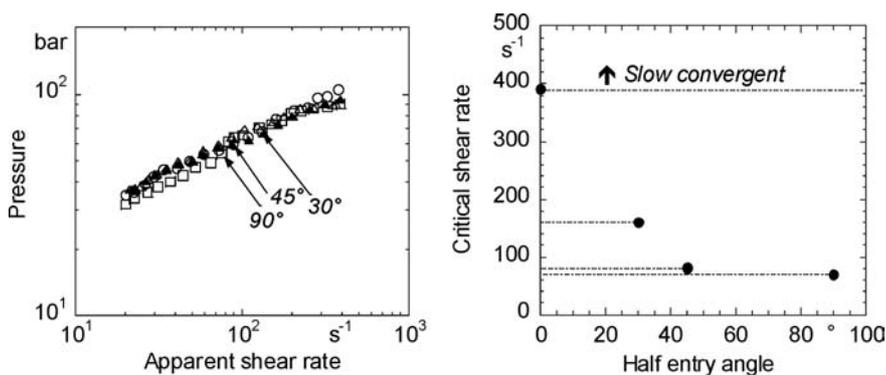
Fig. 33. (a) Apparent flow curves for the different entry half-angles, at a temperature of 180 °C. Arrows indicate the onset of volume instability. ( $L = 20.75$  mm,  $\blacktriangle = 30^\circ$ ,  $\bullet = 45^\circ$ ,  $\square = 90^\circ$ ). (b) Critical apparent shear rate as a function of convergent entry half-angle, at a temperature of 180 °C (For details see Combeaud et al. [72])
