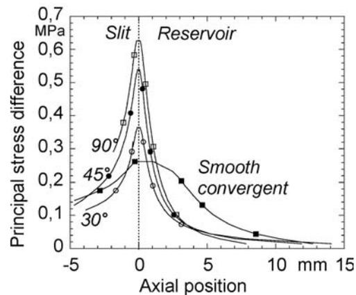
Fig. 32. Centre line principal stress difference measurements for different entrance geometries (For details see Combeaud et al. [72])
