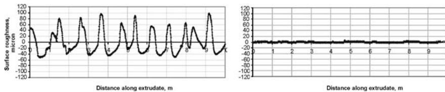
Fig. 12. Effect of additive on sharkskin surface instability for same extrusion conditions. Data on the left hand side additive free, data on the right hand side for polymer containing 1500 ppm fluoropolymer processing aid (For details see Arda and Mackley [7])
