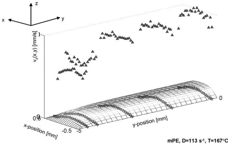
Fig. 21. Velocity profiles and matching numerical simulation in stick-spurt region of flow for mPE (For details see Robert et al. [40])
