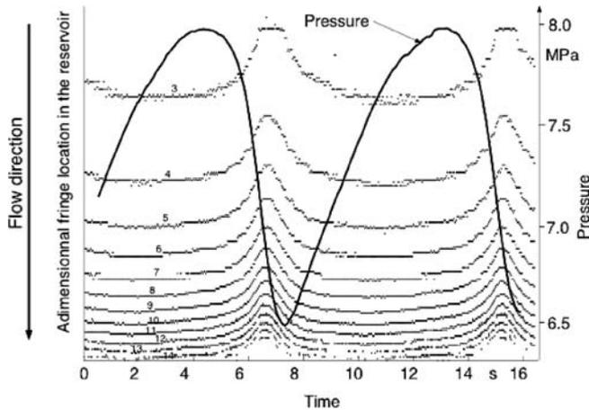
Fig. 23. Reservoir pressure and centre line birefringence variation as a function of time during stick-spurt. The fringe numbers increase from 3 to 14 from upstream of the die entry towards the contraction (For details see Robert et al. [39])
