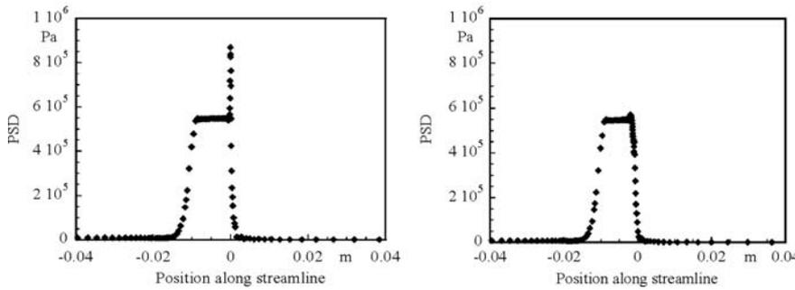
Fig. 11. Effect of die exit curvature on the observed stress field at the exit of a slit flow and also the prediction of Principal Stress Difference profiles along a streamline 50  $\mu\text{m}$  from the slit wall and free surface (For details see Arda and Mackley [7])
