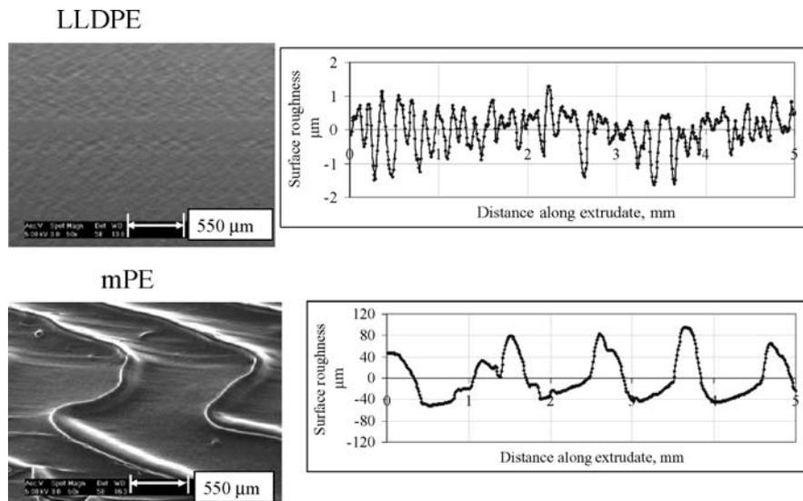
Fig. 3. Examples of sharkskin SEM and surface roughness profiles for LLDPE and mPE (For details see Arda and Mackley [7])
