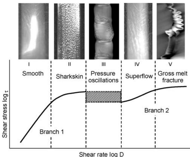
Fig. 1. Examples of different forms of extrusion instabilities seen for linear polyethylene (For details see Merten et al. [21])
