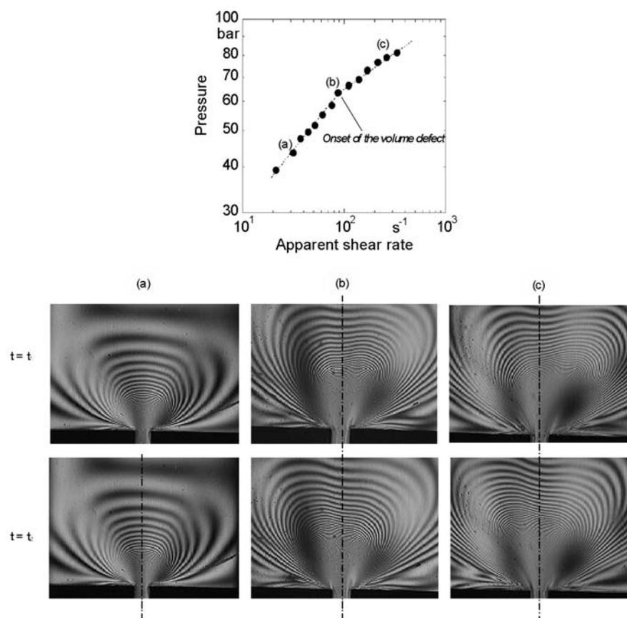
Fig. 29. Apparent flow curve and associated FIB patterns (a):  $30 \text{ s}^{-1}$ , (b):  $87 \text{ s}^{-1}$ , (c):  $263 \text{ s}^{-1}$  (abrupt contraction,  $T = 180^\circ\text{C}$ ,  $L = 25 \text{ mm}$ ,  $H = 1 \text{ mm}$ ) (For details see Combeaud et al. [72])
