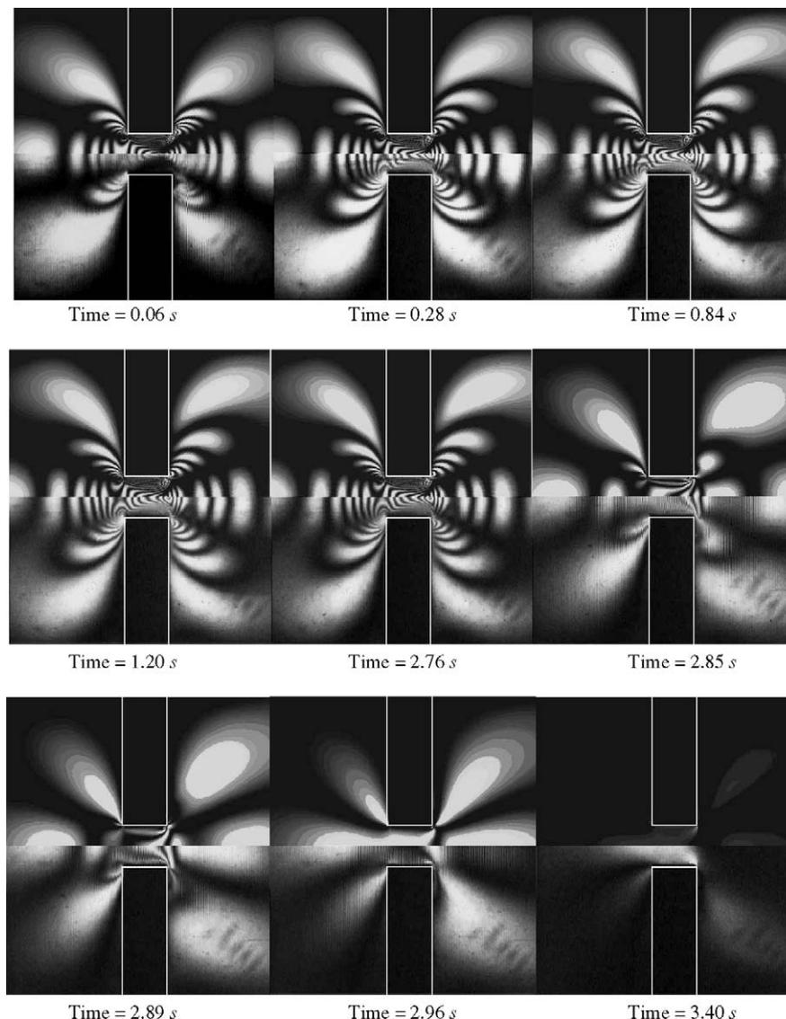
Fig. 2. MPR4, matching of time dependent simulation (top) with experiment (bottom) for LLDPE at 185 °C for a piston speed of 5 mm/s. Flow is from left to right in the figure, slit geometry is drawn in white on the pictures. Rolie Poly simulation with compressible flow.
