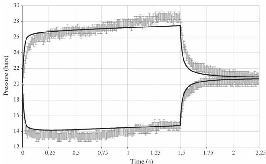
Fig. 4. Time dependent absolute pressure profiles for MPR2, LLDPE at 185 °C at a piston speed of 4 mm/s. Experimental data (error bar I) for both top (top curves) and bottom (bottom curves) piston, matching numerical simulation (—) for compressible Rolie Poly model.
