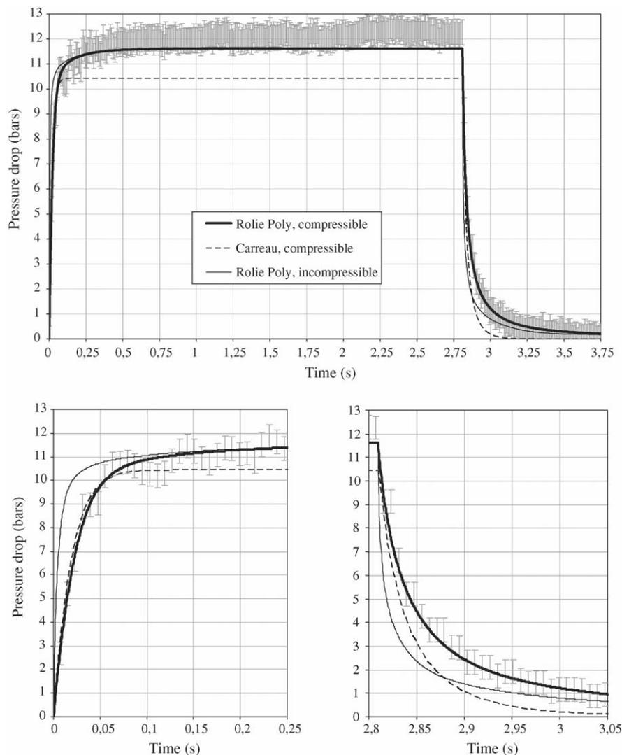
Fig. 3. Time dependent pressure difference profile for MPR4, LLDPE at 185 °C at a piston speed of 5 mm/s, complete curve (top) and details of start up (bottom left) and relaxation (bottom right) flow. Experimental data (error bar I), compressible Carreau (---), incompressible Rolie Poly (—) and compressible Rolie Poly (—).
