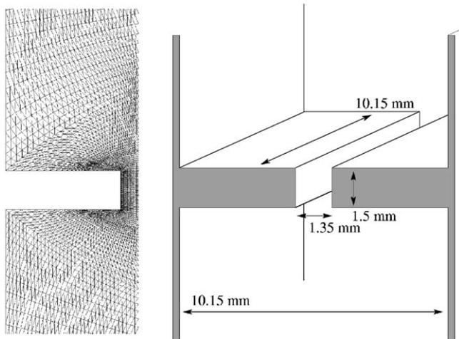
Fig. 1. Detail of the two-dimensional numerical grid and schematic diagram of the slit experimental geometry (gap,  $h = 1.35$  mm, length,  $L = 1.5$  mm, and width,  $W = 10.15$  mm) that was used in both MPR2 and MPR4 experiments.
