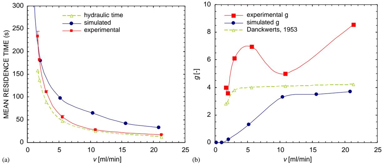
Fig. 8. Effect of net flow rate over (a) tracer mean residence time and (b) backmixing,  $g$ , assuming a perfect step input at steady flow (no fluid oscillations). A comparison is presented between experimental (■) and simulated values (●) using a 2D-axisymmetric model.
