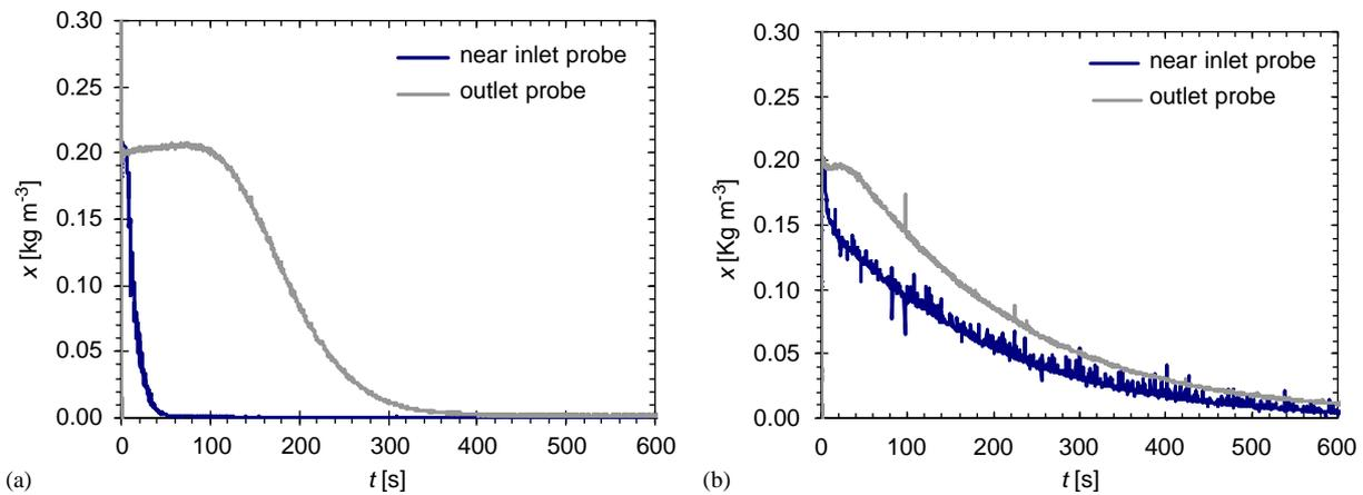
Fig. 5. Experimental  $C$ -curves (tracer concentration along experimental time) at a point near the inlet and at the outlet of a SPC tube at: (a) 3 Hz and 0.5 mm; (b) 20 Hz and 3.0 mm. Net flow rate of 1.94 ml/min.
