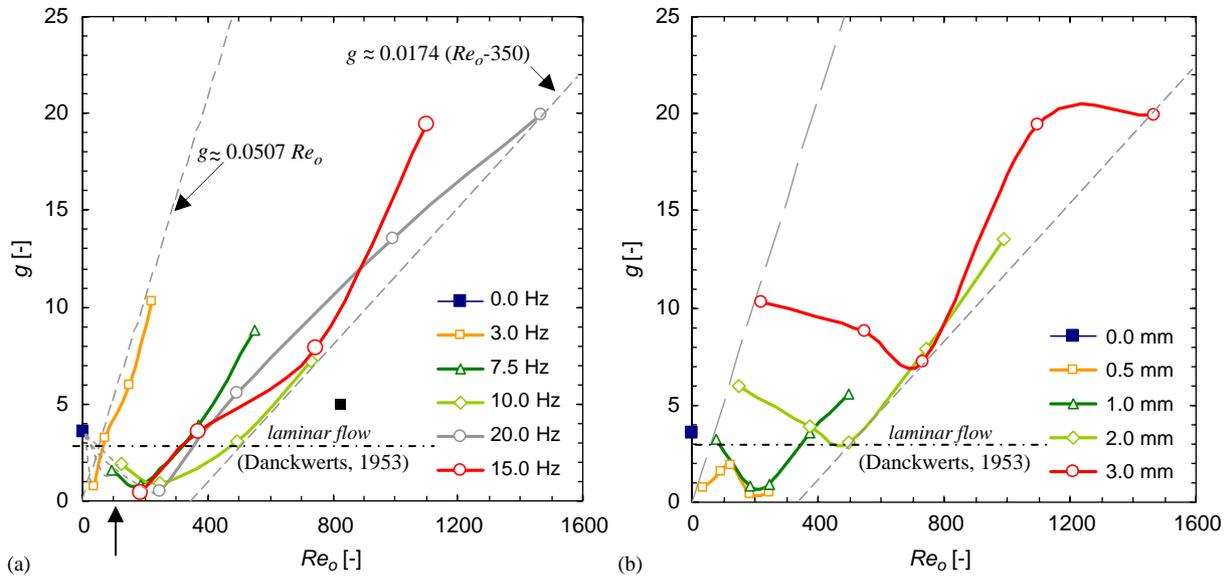
Fig. 7. Fitted backmixing parameter  $g$  using Laplace transforms as a function of  $Re_o$  at: (a) various  $x_0$  and (b) various  $f$ . All values were obtained considering a perfect pulse input, a flow rate equal to 1.94 ml/min and a number of stages equal to 26.
