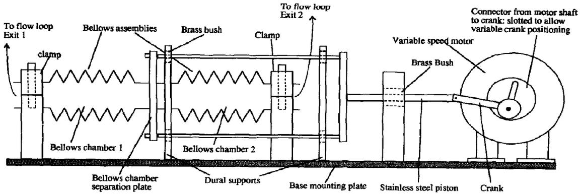
Fig. 1(b). Schematic diagram of oscillating bellows assembly.
