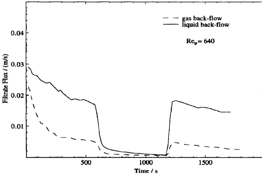
Fig. 7. Filtrate flux vs time: liquid and gas back-flow.
