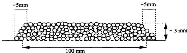
Fig. 4. Schematic diagram of a filter cake formed in steady flow.
