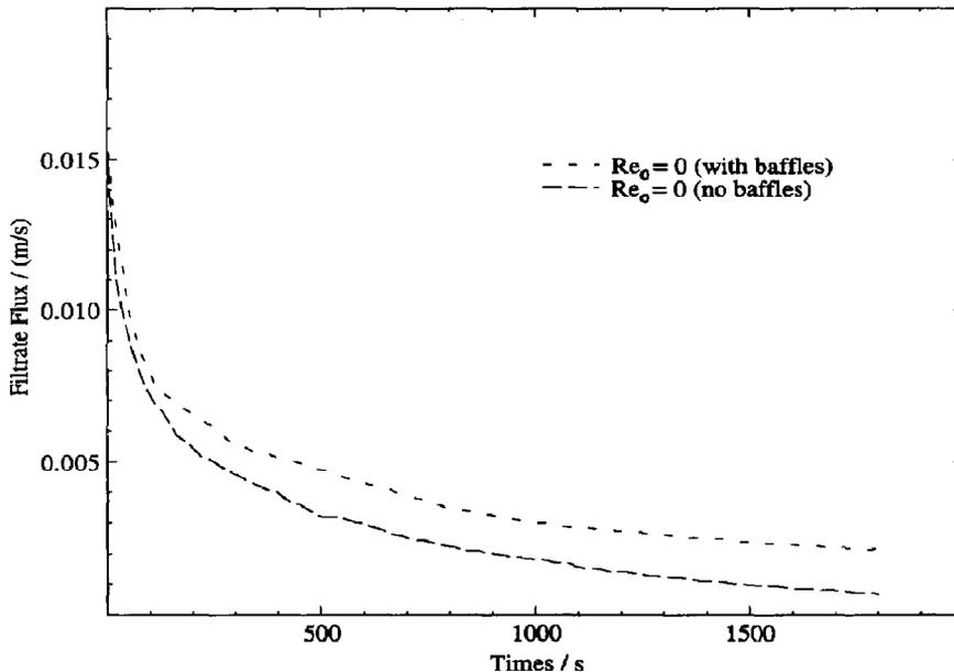
Fig. 3. Filtrate flux vs time: steady flow.  $Re_n = 450$ .
