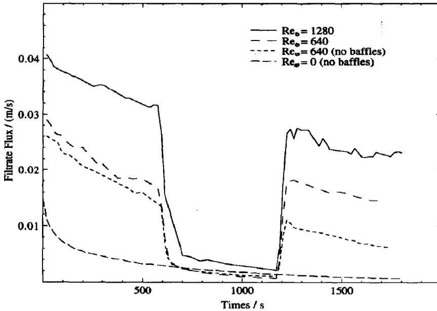
Fig. 6. Filtrate flux vs time: oscillatory flow.
