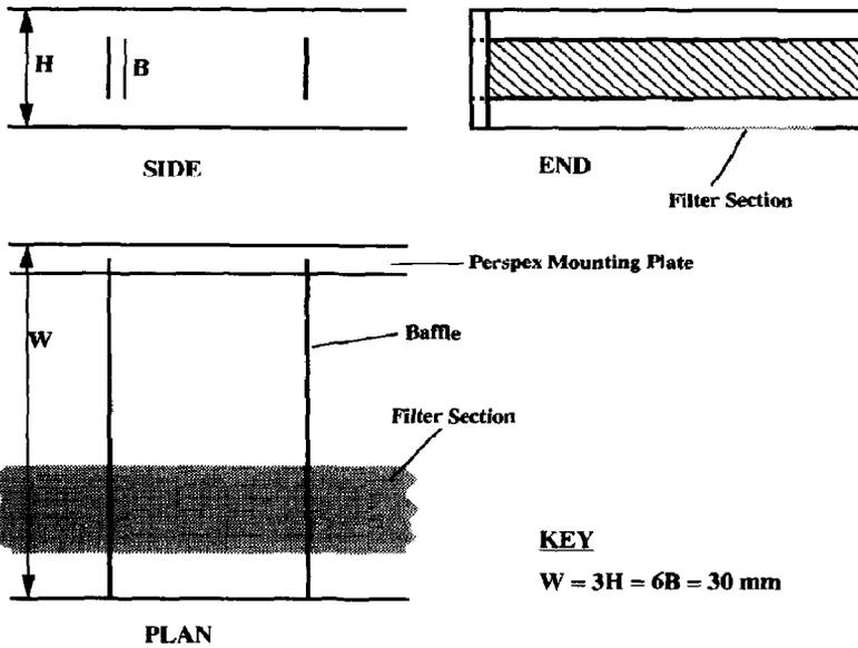
Fig. 2. Schematic diagram of the baffled channel.
