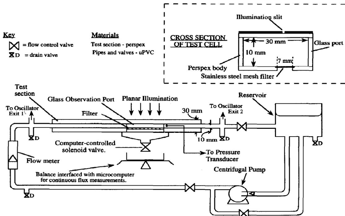
Fig. 1(a). Schematic diagram of the flow loop and test cell.
