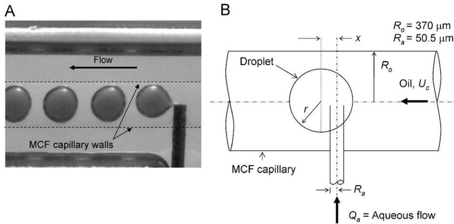
**Fig. 8.** (A) Photomicrograph of droplet formation, illustrating the typical manner in which drops detach from the injecting needle and (B) schematic diagram illustrating theoretical droplet growth and motion away from the injecting needle during formation.
