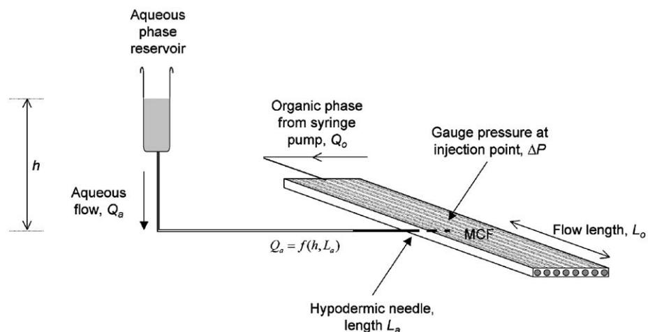
Fig. 4. Schematic diagram illustrating the dependent variables controlling the aqueous phase flow-rate.
