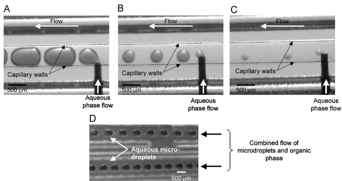
Fig. 3. Photomicrographs illustrating: (A) microslug formation at high aqueous phase flow rates and low organic phase flow rates, (B) medium-size microdroplet formation at comparable organic and aqueous phase flow rates and (C) formation of small microdroplets at high organic phase flow rates and low aqueous phase flow rates. Also shown in (D) is a proof-of-concept for simultaneous microdroplet formation in multiple capillaries.
