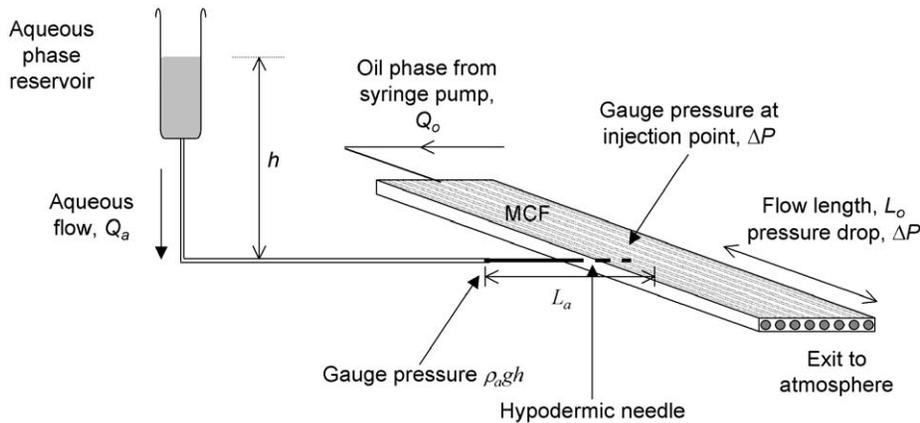
Fig. 7. Schematic diagram of the pressure balance used to calculate the aqueous (disperse) phase flow-rate and the pressure at the tip of the needle that introduces this phase.
