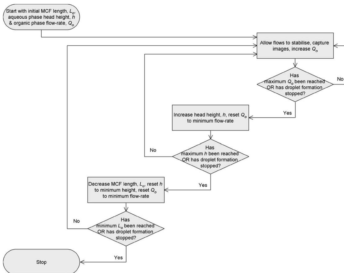
Fig. 5. Flow chart illustrating the 'nested' structure of the experimental protocol.
