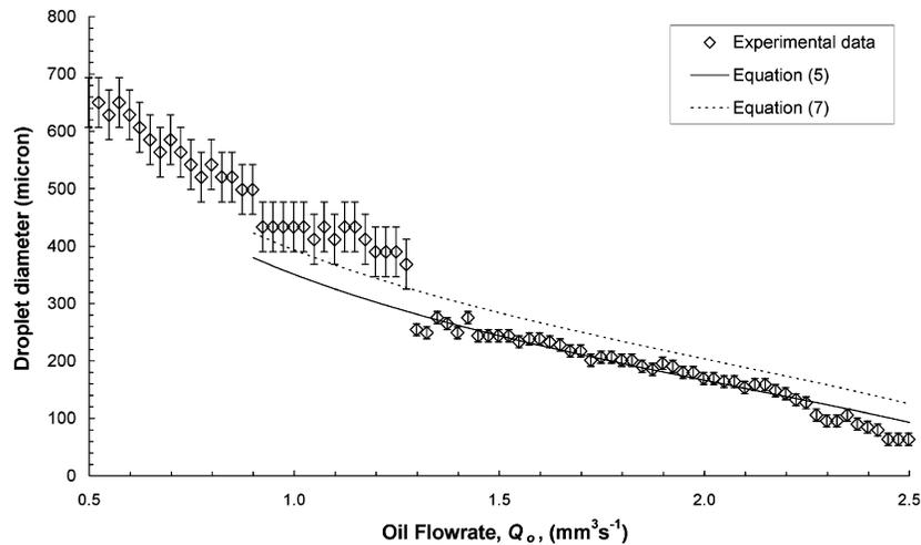
**Fig. 9.** Plot of the observed experimental droplet diameter (open diamonds) as a function of organic phase flow rate. The theoretical curves used Eq. (2) to get  $Q_a$  and  $r_d$  from Eqs. (5) and (7), with  $U_c = 2Q_o/\pi R_o^2$ . Values used:  $R_a = 50.5 \mu\text{m}$ ,  $R_o = 370 \mu\text{m}$ ,  $L_a = 19.1 \text{ mm}$ ,  $L_o = 0.27 \text{ m}$ ,  $h = 0.718 \text{ m}$ ,  $\mu_a = 0.001 \text{ Pa s}$ ,  $\mu_o = 0.067 \text{ Pa s}$  and  $\rho_a = 994 \text{ kg m}^{-3}$ .
