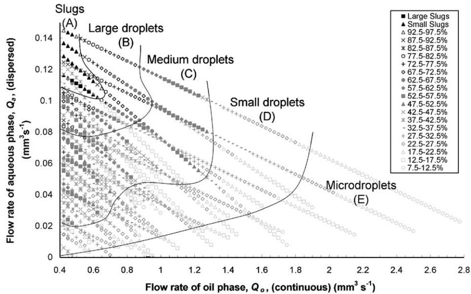
Fig. 6. Plot of droplet diameter expressed as a percentage of capillary diameter as a function of aqueous and organic phase flow rates.
