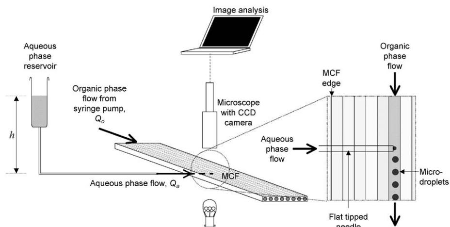
Fig. 2. Schematic diagram of the experimental equipment used to generate microdroplets.
