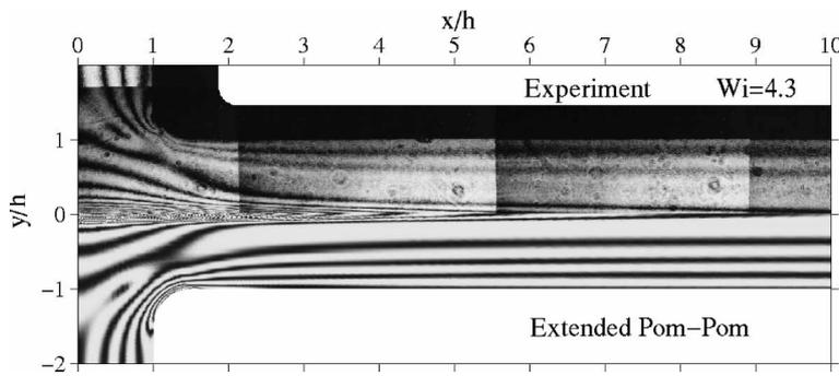
Fig. 5. Measured (top) and calculated (bottom) isochromatic fringe patterns for the extended Pom-Pom model at  $We = 4.3$  of LDPE, DSM Stamylan LD 2008 XC43,  $T = 150\text{ }^\circ\text{C}$ ,  $lcn = 3.4294\text{ [s]}$ ,  $u2D = 3.1\text{ [mm/s]}$ , see [12, 24] for further details
