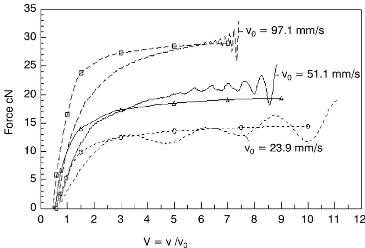
Fig. 6. Comparison of experimental (lines) and simulation (lines with symbols) for Rheotens curves of HDPE, DSM Stamylan, HD8621 for various flow rates, die  $L/D = 15$  ( $50\text{ }^\circ\text{C}$ ), see [35] for further details
